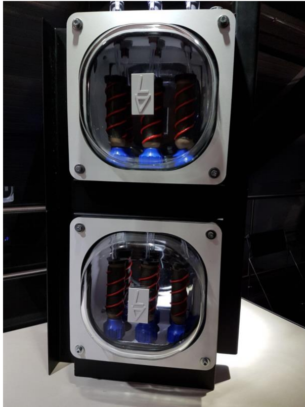
Figure 4: First test prototype 1 for a Microbial Fuel Cell, vertically and horizontally stackable modular building element. Credit: Living Architecture Consortium, photo: LIQUIFER Systems Group, 2017
